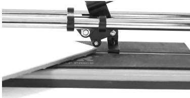
Slide the wheel forward by pushing the handle down with medium pressure.
