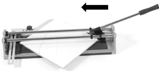
Put tile on the machine against the adjusted angle ruler.
