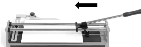
Place the cutting wheel on the rear edge of the tile.
