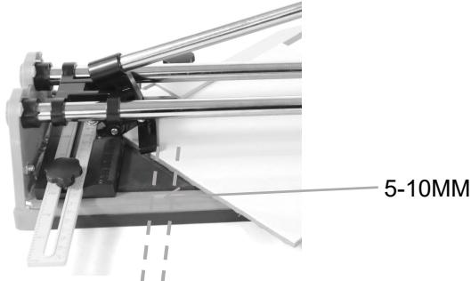
Tips: After scoring, it is better to pull back the handle to let the breaker slightly backtrack 5-10mm,it's the best position to break the tile.
