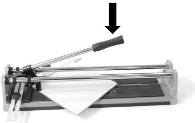
After scoring and without moving the tile position, so that the breaker is slightly in the front edge of the tile and front stop.
