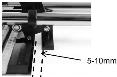
Tips: After scoring, it is better to pull back the handle to let the breaker slightly backtrack 5-10mm,it's the best position to break the tile.
