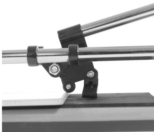
Slide the wheel forward by pushing the handle down with medium pressure.
