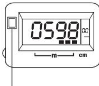
**Press the reset button to reset the counter**
