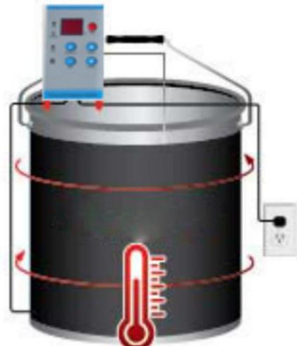
Insert controller probe between the blanket and bucket Set controller to desired temperature range.
