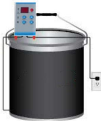
If using with a controller, plug blanket into controller and plug the controller into the power source.
