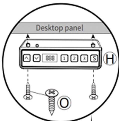
The controller can be fixed to the tabletop
