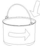
**Step 3.** Put the removable bowl into the machine and slightly turn around the bowl to make it fitted well with the fixed bowl (See below picture).
