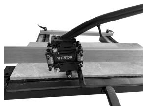
Place the cutting wheel on the rear edge of the tile.
