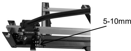
Tips: After scoring, it is better to pull back the handle to let the breaker slightly backtrack 5-10mm, which is the best position to break the tile.
