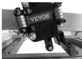
Slide the wheel forward by pushing the handle down with medium pressure.
