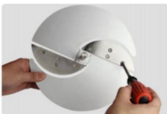
4、Remove blade with screwdriver, Removed blade.
