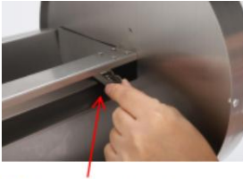
SL-02 Remove the safety buckle by hand to remove the cutter head.
