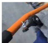
16. Install the throttle switch
