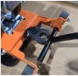
7. The crossbar is inserted into the machine bracket
