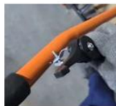
16. Install the throttle switch
