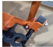
12. Securely tighten the anchor cap
