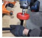
6. Tighten the gasket bolt
