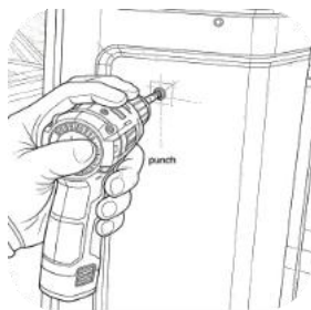
Drill holes based on the determined installation location.
