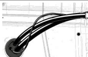
Run the piping and wiring harness into the cab the rubber sleeve is fixed at the opening
