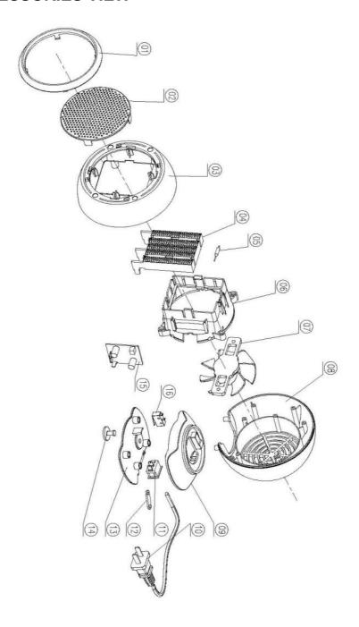
1.Declaration Ring 2.Grille 3.Front Body 4.PTC 5. Thermal Cut-out 6.PTC Support 7.DC Motor 8.Back Body 9.Basement 10.Power Cord 11.ON/OFF Switch 12.Press Board 13.Basement Cover 14.Pole
