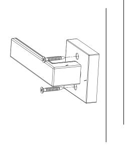
Insert the two screws and tighten the inner plate on the door firmly.
