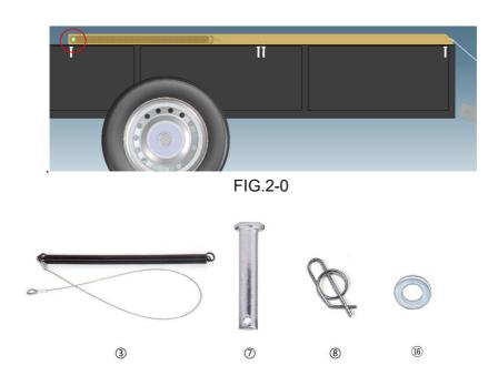
1) Slide a spring/cable assembly into housings A & B. The pin A ⑦ passes through the springs loop (two springs loop) and housings A, as
