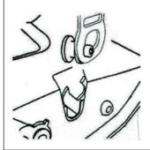
When the Bed Extender is at the furthest rear position. Push down on the the buckle to insert it into tailgate latch. Tighten straps. To release, pull the tailgate handle.
