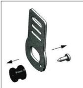
Remove the Screw with a Philips Head driver.
