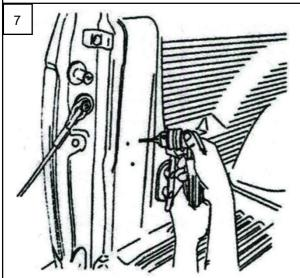
Use a power drill and  $\,\Phi\,4.1\,$  drill bit to drill through the sheet metal. If equipped with a bed liner, drill through the bed liner as well.
