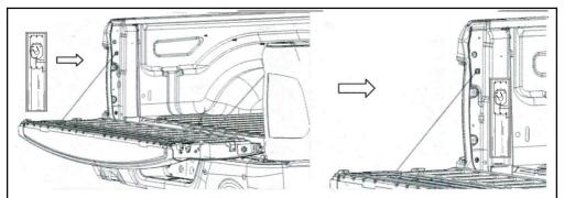
Adjust and place the drilling template Q at the tailgate D-pillar and mark the 3 screw holes with marker on both sides
