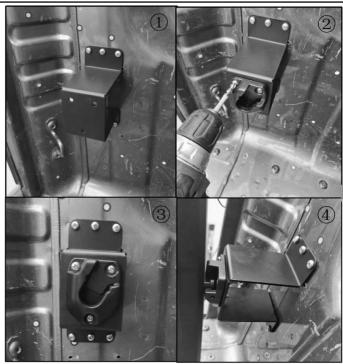
Use a power drill and  $\ \ \phi$  4.1 drill bit to drill through the sheet metal. If equipped
