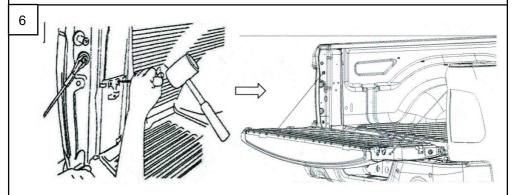
Use the center punch to mark screw holes for preparation of drilling.
