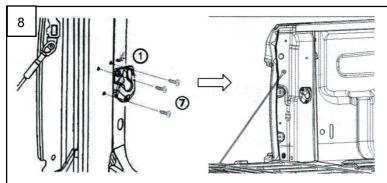
Fasten Bracket D with Screw H by using a Phillips screw
