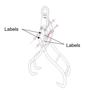
Note: The screws cannot be locked to the point that they cannot be loosened, and the activity space of the linkage parts needs to be reserved.
