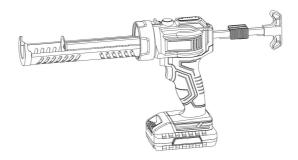
To remove the 300ml cartridge barrel, slightly pull the barrel replacement switch backward, at the same time rotate barrel by 90 ° and pull it out.
