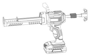
To install 600ml cartridge barrel, rotate barrel directly.
