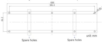
Step 2.Make Holes in the wall with a drill, and insert the dowels into the holes by using hammer.
