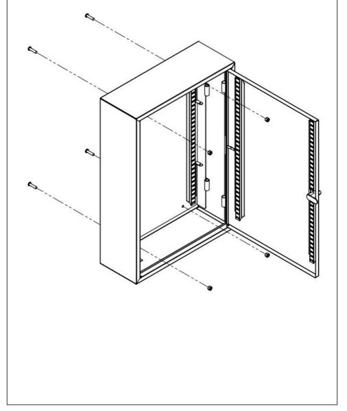
Align the hole positions of the separator plate and the Cabinet, Thread the M6 bolts through the holes and screw on the nuts that disassembled in step1.
