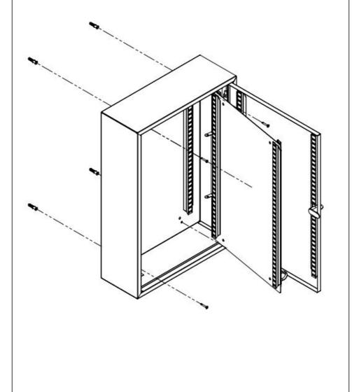
Install the Hangers segments on the cabinet. First the long side then the short.
