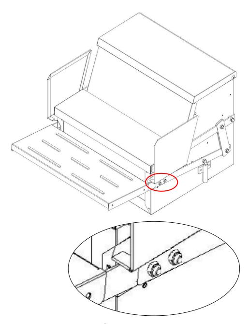
Lock the screws with **2**4-M4 nuts.
