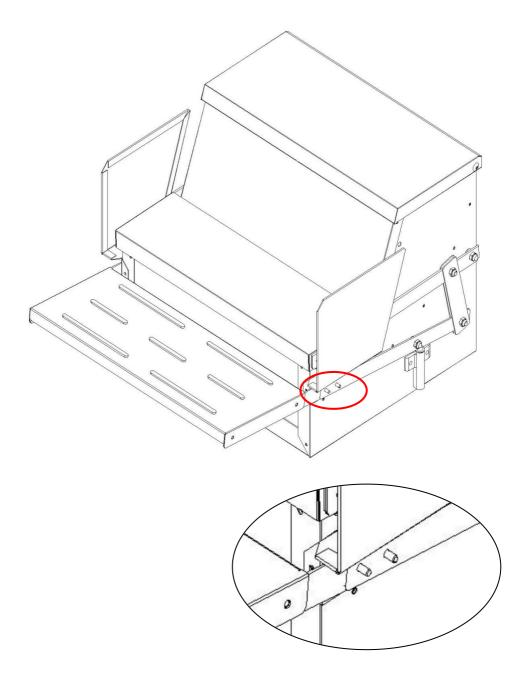
Align the 4 posts of pedal B and the hole positions of body A to assemble.
