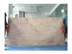
4.After the transportation process is completed, put down the materials and hold, then the mouth of the device will be open, so that you can remove the device.
