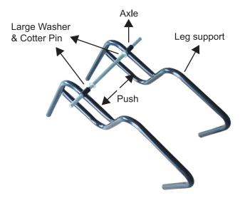
**Step 5:** Attach the wheel to the axle with a large washer and cotter pin.
