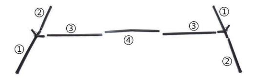
**STEP 2:** Slip one side net sleeve over one of the fiberglass poles. Insert the the same side's base leg post.
