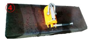
The last step, after confirming that the permanent magnetic lifter is closed, remove the permanent magnetic lifter and store it in a dry place to prevent rust.
