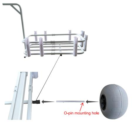
**NOTE:** Insert the plastic parts of the wheel axle into the ends of the bottom cross member of the frame, then insert the wheel axle, and finally install the wheel on it.
