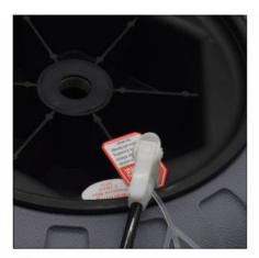
Insert tire valve into top valve of the hand pump. Bend the plastic handle forward to create a seal so that the tire will inflate more quickly.
