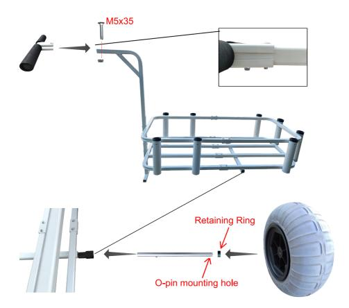
**NOTE:** Insert the plastic parts of the wheel axle into the ends of the bottom cross member of the frame, then insert the wheel axle, and finally install the wheel on it.
