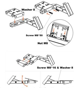
STEP 11: Line up the holes on the Shifter Mounting Arm with the threaded inserts on the vertical post choose your desired height securing with 2x M8\*16mm screws and washers.
