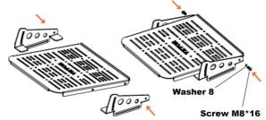
STEP 4: Adjust the pedal plate to your desired angle and bolt through the front holes using 2 x M8\*16 screws and washers.
