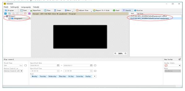
5: The operating panel is shown in the figure. Click the text, graphic and text above the interface to automatically add programs. The show is added to the display screen on the left side of the interface. Right -click on the mouse to add, delete and copy the program.
