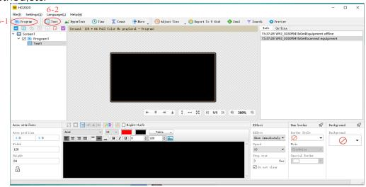
7: Hold the black rectangular orange thread of the mouse can be dragged freely to achieve partitions. After entering the partition text, click to send it. Multiple texts can be displayed on the same display screen
