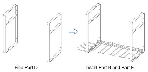
Step 2. Place Part G (Hammer holder), Part F (Pliers holder), and Part B(Groove panel) in the middle layer of t Part D (Bracket), Use the tool Part M (wrench) along with the fasteners Part J (Screw) and Part I (Nut) to securely fasten them in place.
