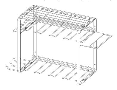
Step 4: Use Part K (Self-tapping screw) and Part L (Dowels) to securely fasten the power tool organizer in the desired location on the wall.
