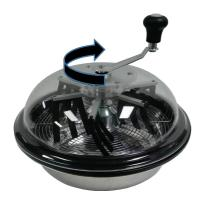
Using the handle, make 15-30 complete turns. While spinning the handle, the inside rubber twist tongues multiply the rate of the spinning plants and blades by over 30 times. A combination of the rubber tongues presses and rolls the plants into the spinning blades can improve the cutting efficiency. Only 30 seconds can yield one hour's work.
