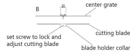
A: To install the cutting blade, first place the blade on the blade collar(Note: the beveled side faces down against the holder collar) and tighten the two-set screw see diagram A.
