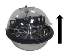
Remove the top from the flower trimmer's base. The inside of the top contains the high-density rubber tong used to push the plant leaves into the blade grill. The cutting blades or wires are located below the grill.
