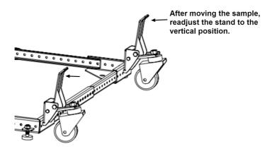
6. Adjust the mobile base to be level by rotating the supporting feet.
