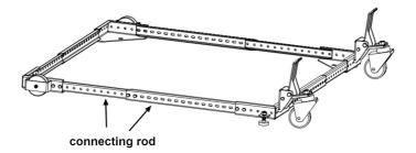
**Note**: To ensure the connection strength, the connection position needs to be fixed with two bolts and nuts, not only one.
