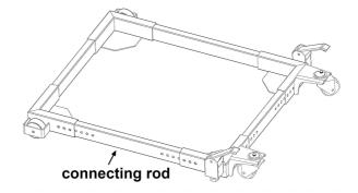
**Note**: In order to ensure the connection strength, the connection position needs to be fixed with two bolts, not only one.
