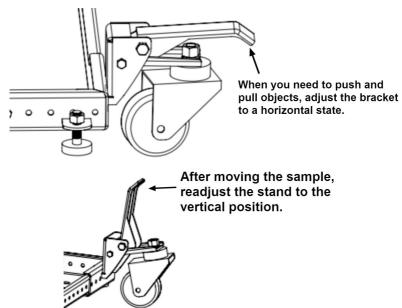
10. Adjust the mobile base to be level by rotating the supporting feet.
