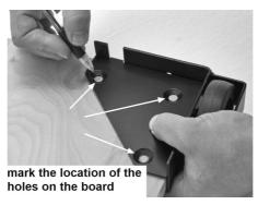
6. Drill the holes using a 1/2 inches drill bit, it is a good idea to check that the holes are lined up to the plate before drilling each hole.
