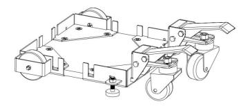
9. Use your feet to move the bracket to the horizontal state to push and pull the object. After moving to the desired position, adjust the bracket to the vertical state again, as shown in the figure below.
