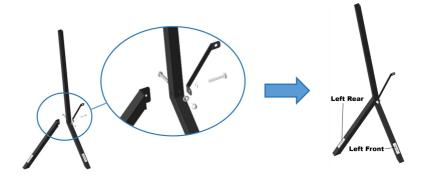
**STEP 2:Assemble right support tube.** (Need M8\*45 1pc、 washer 2pcs and Nut M8 1pc. )
