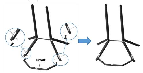
**STEP 5:Assemble the rear connector.** (Need M8\*45 2pcs、 washer 4pcs
