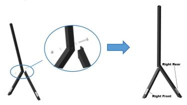
STEP 3:Connect the left and right support tubes. (Need M8\*45 1pc and washer 1pc. )
