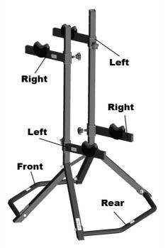
STEP 7:Assemble upper strut and connecting plate.(Need M8\*40 8pcs,
