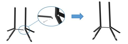
STEP 4:Assemble the front connector. (Need M8\*45  $2pcs_{\smallsetminus}$  washer 4pcs
