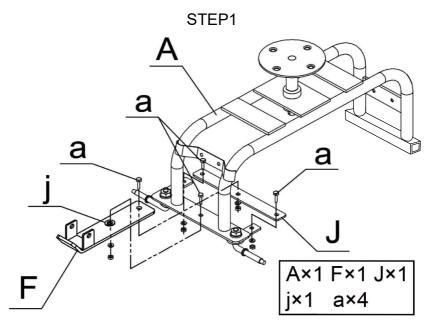
Install the handle controller(F) and steering link connector(J) on the frame(A). NOTE: Loosen half a circle after the screw a(4pcs) tightening to ensure that the handle can turn when used;;
