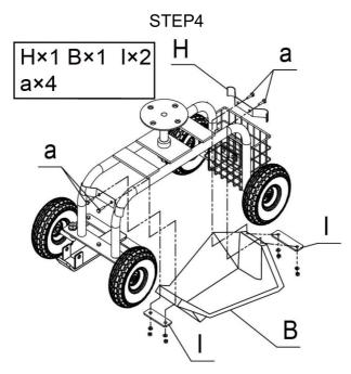
Install the plastic tray(B) on the frame(A).
