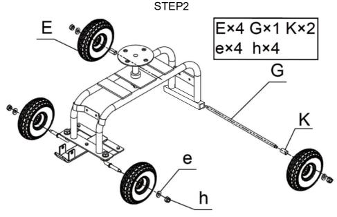
Install four wheels(E) on the frame(A).
