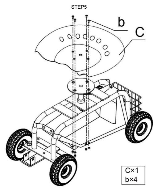
Install the seat(C) on the frame(A).
