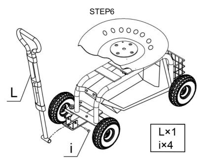
Install the handle(L) on the handle connector(F).
