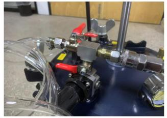
5.Adjust the inlet pressure regulator and rotate clockwise to adjust to the required working pressure, if you want to reduce the pressure in the barrel, rotate in a counterclockwise direction.
