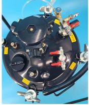
3.Close all valves, the sprayer inlet is connected to the barrel outlet (24), and the sprayer inlet is connected to the barrel outlet valve (12)
