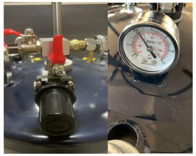
6.Open the outlet valve(12)open the discharge valve(24)
