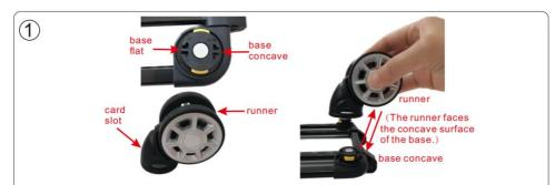
Lay the lever flat, as shown in the figure: The runner faces the concave surface of the base (be sure to pay attention to this), Then press the card slot down hard, and the installation is complete when you hearthe sound of "bang". Ensure that the wheels are properly installed to avoid falling out during use.
