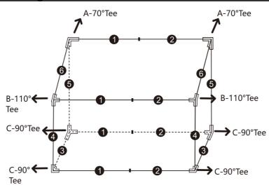
**Assembly Steps** Step1 C-90° Tee\*4 **1** x2 **2**:x2 Put the 1,2 and 3 metal pipes into the bottom of the cloth sleeve after **3**x2 assembly according to the legend. Step2 A-70° A-70°Tee **€** Tee B-110°Tee **→**B-110° A-70° Tee Tee×2 B-110° Tee×2 **1**x2 **2**:x2 **4** x2 **5**x2 Outfall Vent **6**x2 Assemble other metal pipes in turn. Step3
