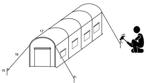
Tied the string in the back of the cover to the frame.Use the ropes and stakes for four corners of the greenhouse, to reinforce the stability of it.
