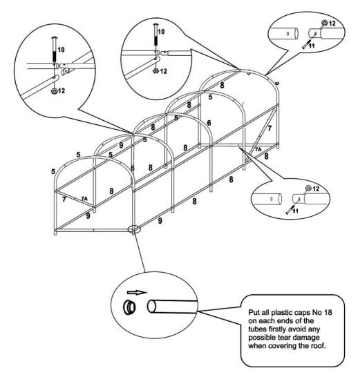
Loosely assemble completed frame before tightening all bolts in final position.
