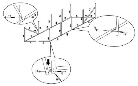
Loosely assemble complete frame, before tightening all bolts in final position.
