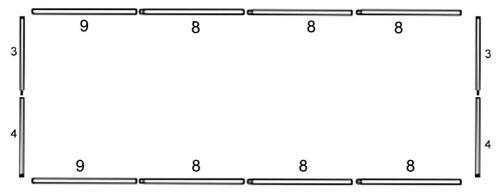
Assemble for 2 sets floor tubes No3+ No4 use the shorter bolts, and the horizontal frame No9+No8+No8+No8 together.
