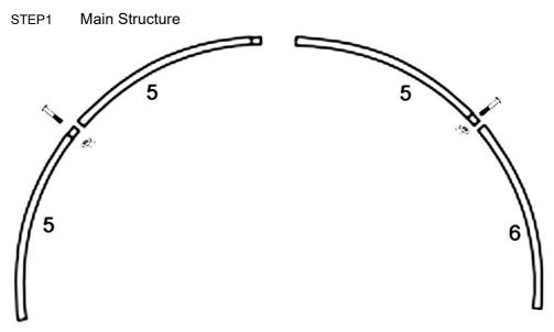
Assemble each 4 sets No.5+No.5 together, make them into one part first, use the shorter bolts, put the curve tube on the flat ground, make both tubes horizontal, then tighten the nuts. And assemble for 4 sets No.5+No.6 in the same way.
