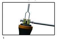
Unscrew both screws on the pen and detach them from the hole where the pen head is installed, making it easier for the pen head to be inserted smoothly to the bottom. The effect is shown in the above picture.
