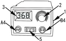
1)Pyrography machine switch: Turn on the switch when using it, and turn it off when not in use to avoid danger.
