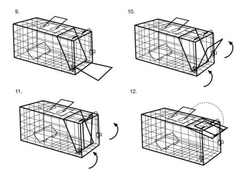
Lift the trap door spring and push towards the bait plate. Now is the time to place the baits behind the bait plate Secure the metal rod using the metal folding tags already attached to the cage.
