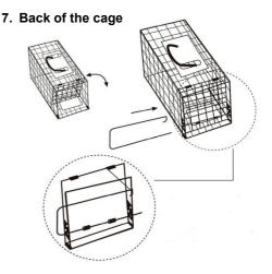
The cage should look like diagram 5. Its currently in an upside down position. Flip and turn the whole cage around so its the correct side up You are now looking at the back of the cage
