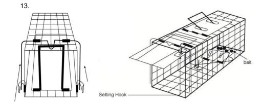
Hold the trap door in an open position, set the trap by swinging the setting hook beneath the bush on the trap door, and then lower the door to release pressure back onto the setting hook. The cage should look like diagram 14. Once set, the trap should be left in position for at least 7 days before relocating.
