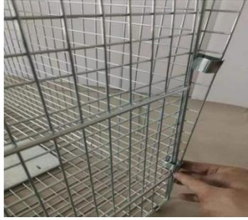
6. Pull out the back door and secure it with a buckle. If you feel that the front and back doors are not secure, use nylon cable ties to reinforce them.
