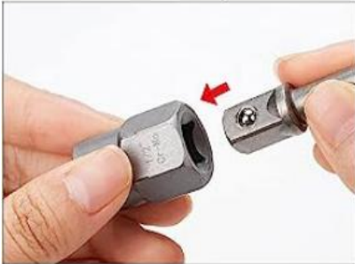
Step 2: Select the required nut extractor size and install it on the connecting rod
