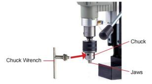
4. Mount your twist drill bit (not included) into the chuck and turn the chuck wrench clockwise until the bit is locked in place.
