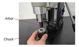
**3.** Loosen the chuck's jaws by inserting the chuck wrench into either hole on the chuck and turning it counterclockwise.
