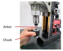
**3.** Loosen the chuck's jaws by inserting the chuck wrench into either hole on the chuck and turning it counterclockwise.
