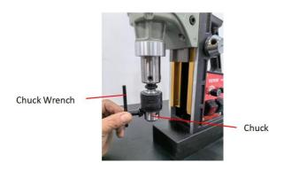
4. Mount your twist drill bit (not included) into the chuck and turn the chuck wrench clockwise until the bit is locked in place.
