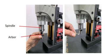
2. Slide the chuck onto the arbor until it is locked into place.
