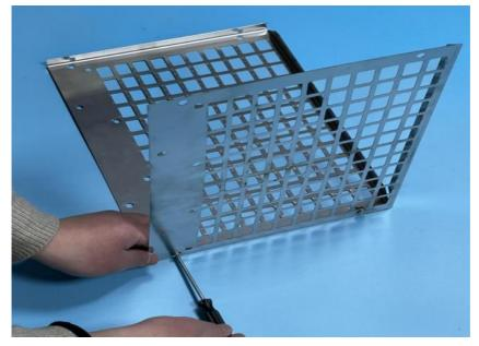
3. Fix the 4 inner reinforced edge strip with screw M5\*8 and flange nut M5.
