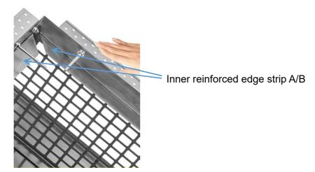
4. Assemble the roof to the 4 coamings with screw M5\*8 and flange nut M5.
