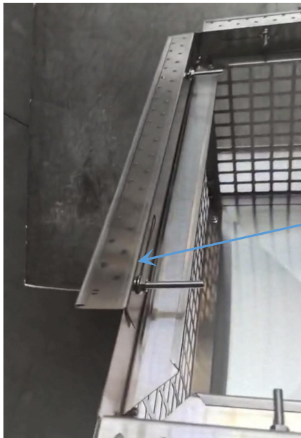
External installation of edge strips A/B
