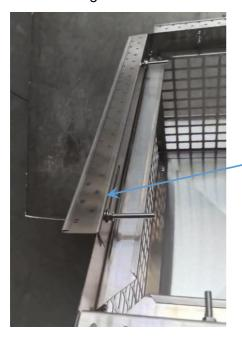
External installation of edge strips A/B
