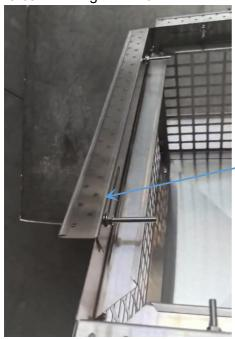
External installation of edge strips A/B
