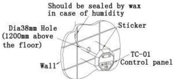
Figure 2 Installation of TC-01 Control panel
